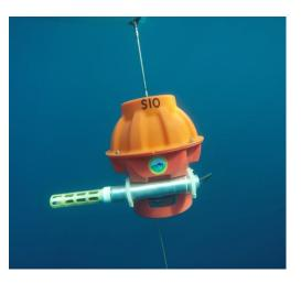
**Deep SOLO** SIO float lab, MRV 0 – 6000 m 25 kg 13" glass sphere SBE-61 CTD Deep NINJA TSK Co LTD, JAMSTEC 0 – 4000 m 50 kg 6' high Extended-depth SBE-41 CTD Oxygen sensor optional
